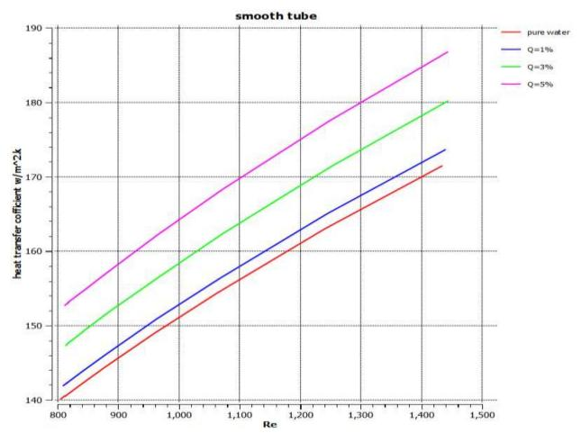
Figure (3): Heat Transfer coefficient Variation with Reynolds Number for the smooth tube with volume concentration (0%, 1%, 3%, 5%)
