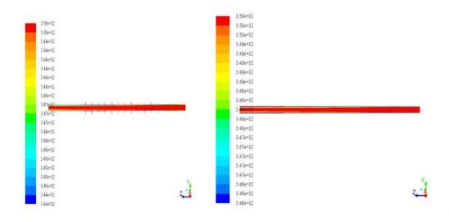
Figure (6): Temperature contours map for AL2O3-Water Nano-fluid (Q=5%) for finned and smooth tube.
