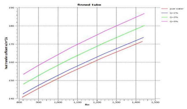
Figure (2): Heat Transfer coefficient Variation with Reynolds Number for the finned tube with volume concentration (0%, 1%, 3%, 5%)
