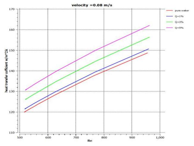
Figure (5): Heat Transfer coefficient Variation with Reynolds Number for the finned tube with velocity = 0.08 m/s and volume concentration (0%, 1%, 3%, 5%)
