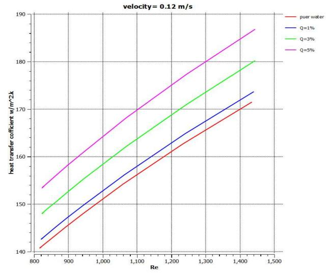
Figure (4): Heat Transfer coefficient Variation with Reynolds Number for the finned tube with velocity = 0.12 m/s and volume concentration (0%, 1%, 3%, 5%)
