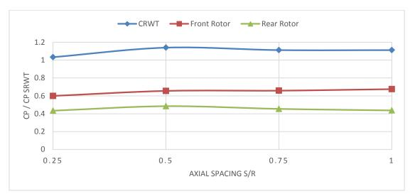
Figure 10:Coefficient of Performance change with axial distance at TSR 4 for front, rear and CRWT versus SRWT at TSR 6
