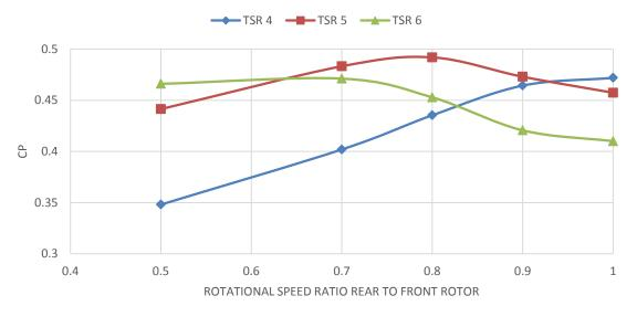
Figure 20:Cp vs rotation speed ratio rear to front rotor at TSR 4, 5 and 6 for CRWT
