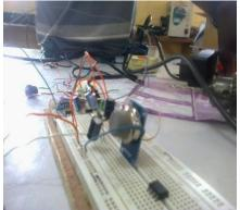
Figure-1.4: Solder-less Experimentation of the Gas Detector
