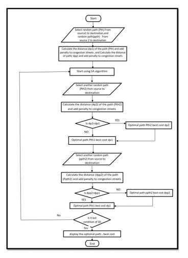
**Fig. 1:** Flowchart for the proposed recommendation module from more than one source node to destination node.
