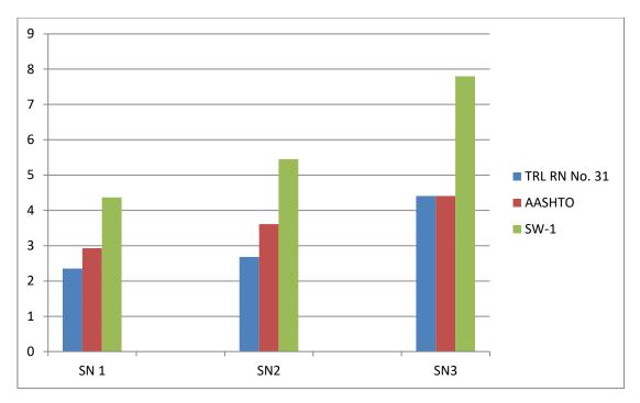
Chart No. (2): The Structural numbers of the obtained Pavement Section
