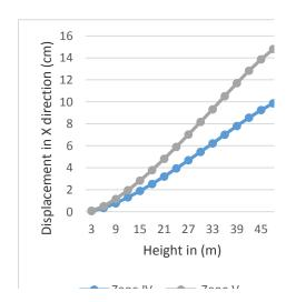
**Figure 16:** Lateral displacement of G+14 building in X direction in zone IV and V.
