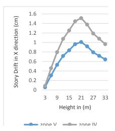
Figure 11: Story drift of G+9 building in X direction in zone IV and V.
