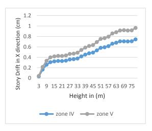
**Figure 29:** Story drift of G+24 building in X direction in zone IV and V.
