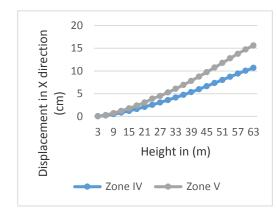
Figure 22: Lateral displacement of G+19 building in X direction in zone IV and V.
