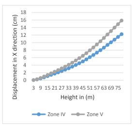
Figure 28: Lateral displacement of G+24 building in X direction in zone IV and V.
