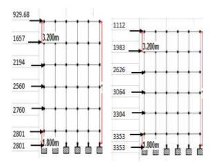
**Figure 7:** Base shear of G+4 building in X and Z direction in zone IV and V.
