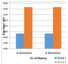
Figure 6: Base shear of G+4 building in X and Z direction in zone IV and V.
