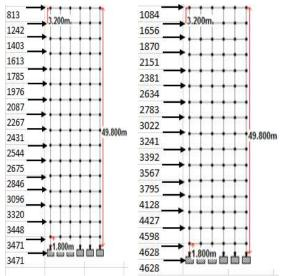
Figure 19: Base shear of G+19 building in X and Z direction in zone IV and V.
