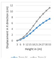
Figure 10: Lateral displacement of G+9 building in X direction in zone IV and V.
