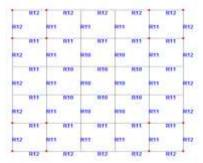
Figure 31: Column orientation which lie in corners of G+4, G+9 G+14, G+19 and G+24 in Zone IV and V
