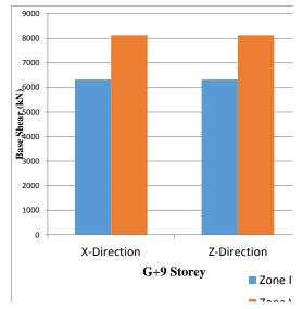
Figure 12: Base shear of G+9 building in X and Z direction in zone IV and V.
