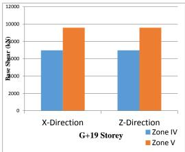
**Figure 24:** Base shear of G+19 building in X and Z direction in zone IV and V.
