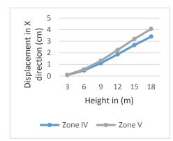
Figure 4: Lateral displacement of G+4 building in X direction in zone IV and V.
