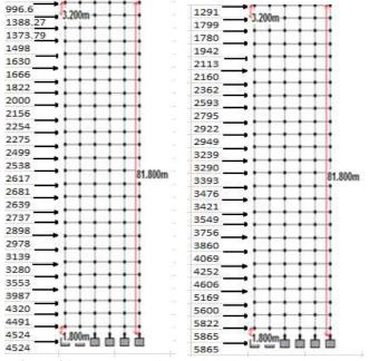
Figure 31: Base shear of G+24 building in X and Z direction in zone IV and V.
