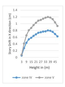
**Figure 17:** Story drift of G+14 building in X direction in zone IV and V.
