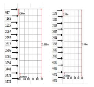
Figure 13: Base shear of G+9 building in X and Z direction in zone IV and V.
