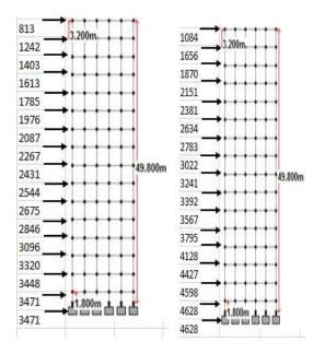
Figure 25: Base shear of G+19 building in X and Z direction in zone IV and V.
