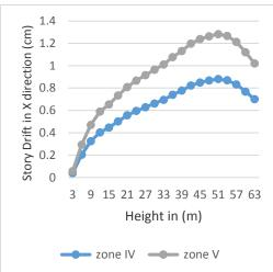
Figure 23: Story drift of G+19 building in X direction in zone IV and V.
