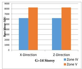
Figure 18: Base shear of G+14 building in X and Z direction in zone IV and V.
